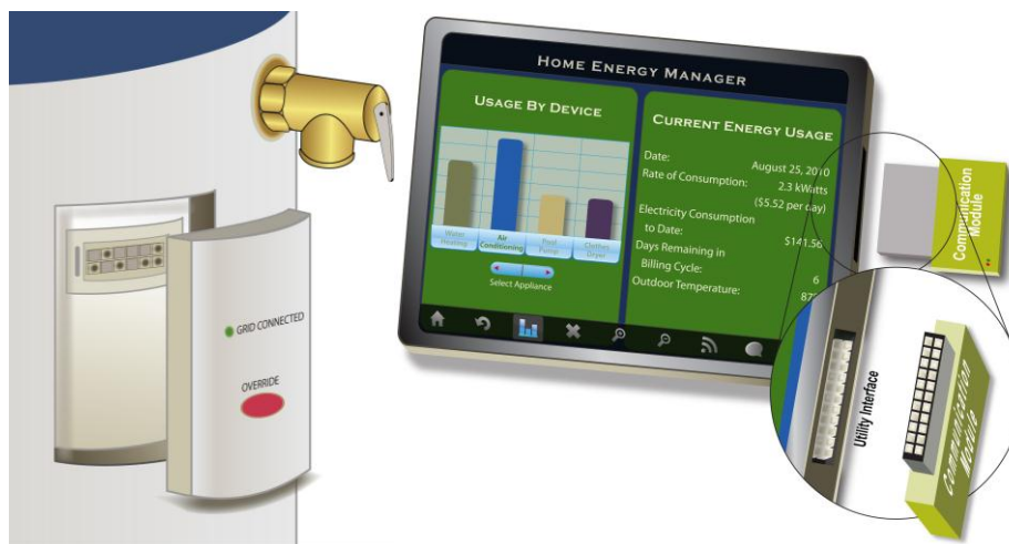
Figure 2-1 – Illustrations of the Modular Communications Concept on a controlled device (left) or Energy Management Console (right)
